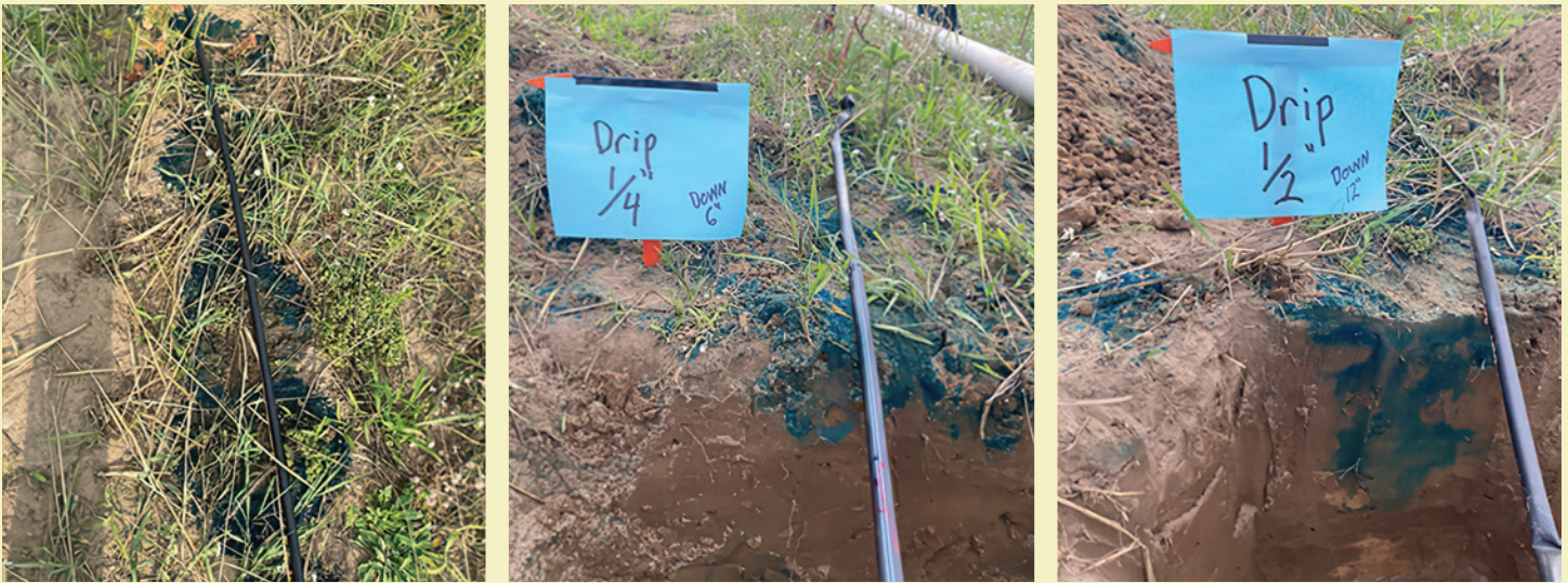
Figure 5 – Blue dye demonstration to show the water flow in soil caused by different irrigation amount.
