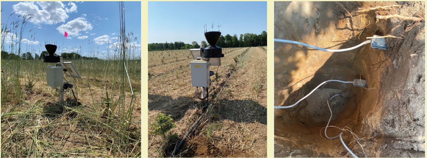
Figure 2 – Installed IoT-based Sensor Monitoring System in Christmas Tree Farms (left and middle). Installed Soil Moisture Sensors at 6-, 12-, and 24-inch Depth (right).
